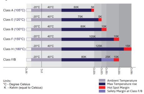
**Hot spots** are areas on the windings where the temperature rise is highest, leading to greater heating of insulation materials. To ensure protection in these regions, lower temperature limits are set for the insulation.
