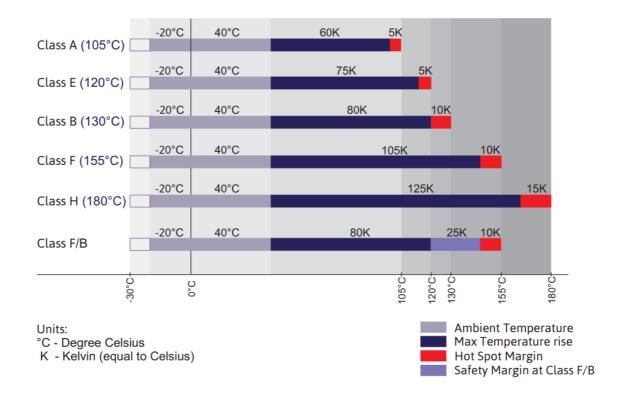
The maximum permissible temperature rise of the winding is determined based on the thermal class temperature limits. The temperature of the winding increases as a result of the copper and iron losses in the electric motor during operation. The winding temperature rise is determined through measuring the winding resistance, which increases with increasing temperature. To allow for any Hot Spots in winding lower temperature limits are specified for the insulation materials.
